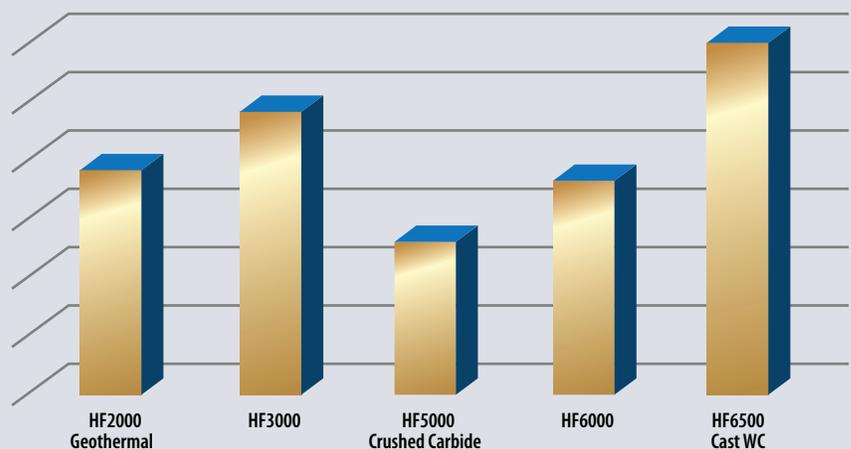
Abrasion testing completed per ASTM G65 – 16 using the dry sand/rubber wheel test method and quantitative values determined from adjusted weight loss.
