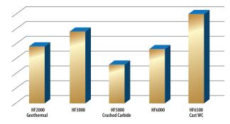
Abrasion testing completed per ASTM G65 — 16 using the dry sand/rubber wheel test method and quantitative values determined from adjusted weight loss.
